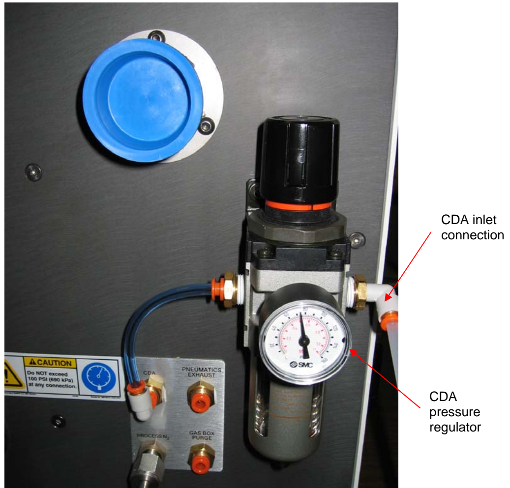
Figure 19. CDA pressure regulator and connection.
