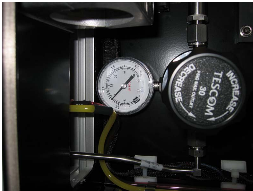
Figure 18. Set N 2 regulator to approx. 10 psi.
