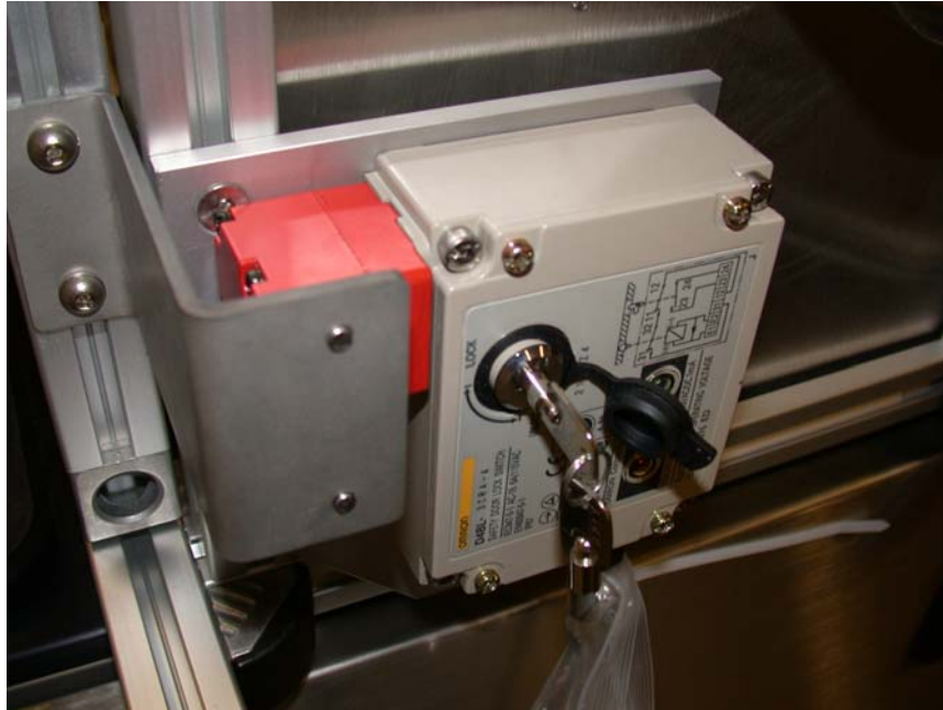
Figure 48. Ventilation shroud interlock with key to override lock.
