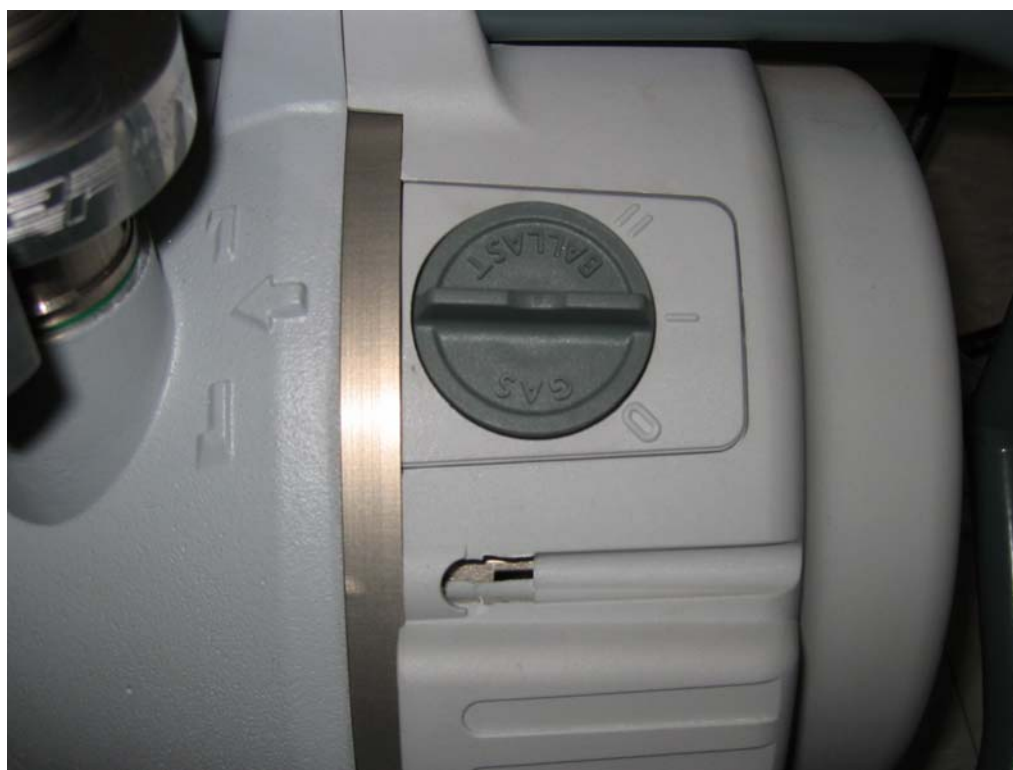
Figure 11. Pump ballast control should be set to position 1.
