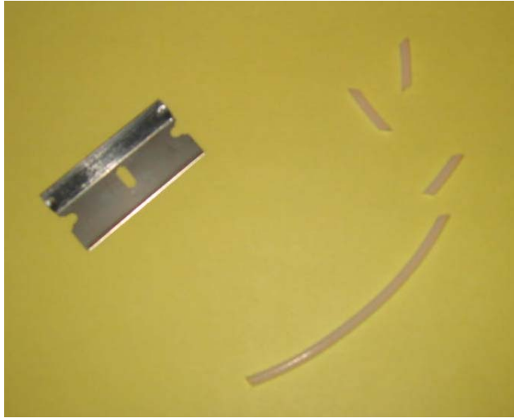
Figure 40. Teflon beading and pieces that have been cut from it using a razor blade.
